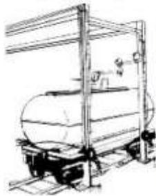
Our clamps are the plier type with sharp, replaceable points. Strong, long-lasting spring enables points to penetrate all paint, rust, etc. You must have bare metal contact to be able to draw off static electricity. The use of Browne ground clamps will allow you to comply with OSHA Standards.
